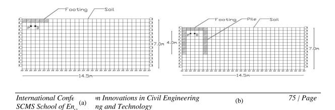
Figure 1 finite element discretization model of footing on soil mass.
